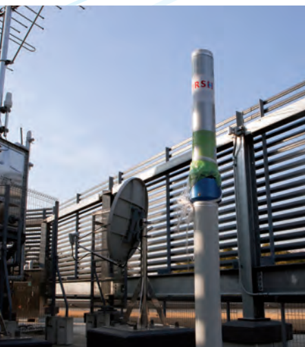
Ambient dose-rate Radiation Protection beacon, installed by IRSN on the roof of the French Embassy
