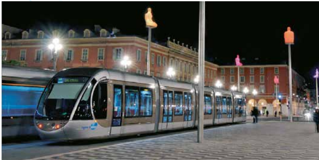
Place Massena: The tram runs on battery power along part of its route.
