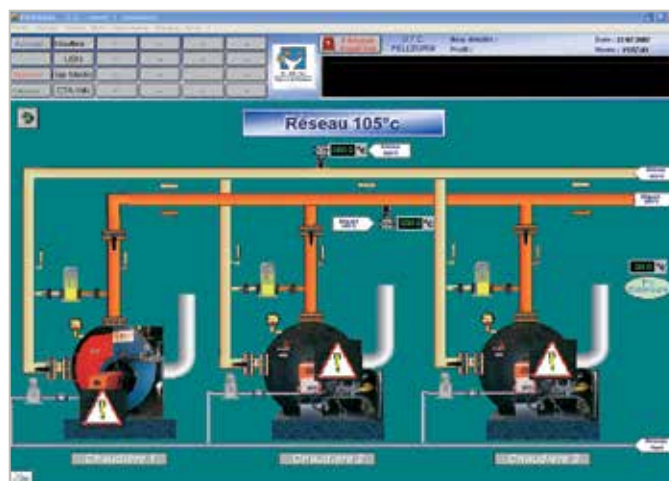
Panorama mimic diagram view for supervising boilers at the Pellegrin hospital.
