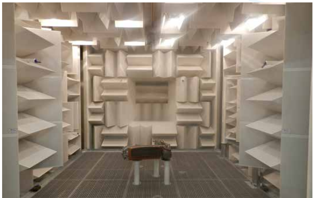
Echo-free chamber for measuring the acoustic environment. Unique in Europe.
